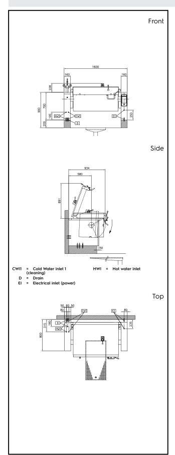
Electric 400 V/3N ph/50/60 Hz Supply voltage: Total Watts: 20.6 kW Installation: FS on concrete base;FS on feet;On base;Standing Type of installation: against wall **Key Information:** Working Temperature MIN: 50 °C Working Temperature MAX: 250 °C Vessel (rectangle) width: 1050 mm Vessel (rectangle) height: 326 mm
